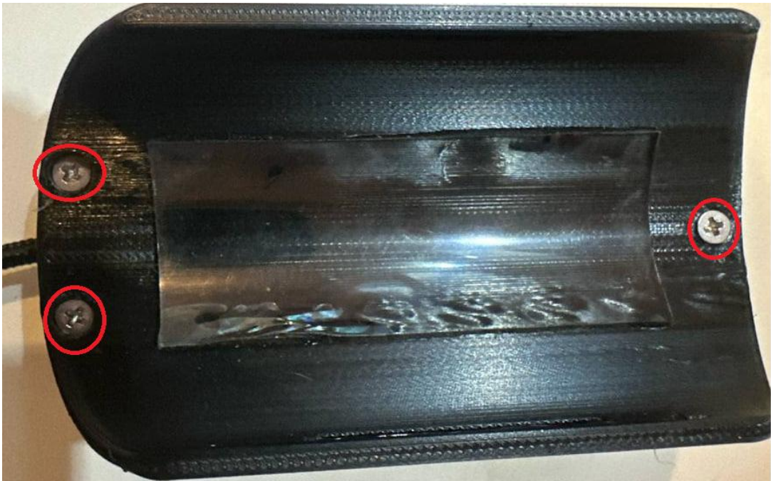
Fig. 14 Joining the two parts of the sensor with screws
