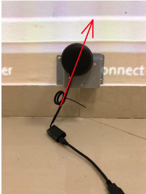
**Pic. 20 Determining the direction of the sensor reference axis**
