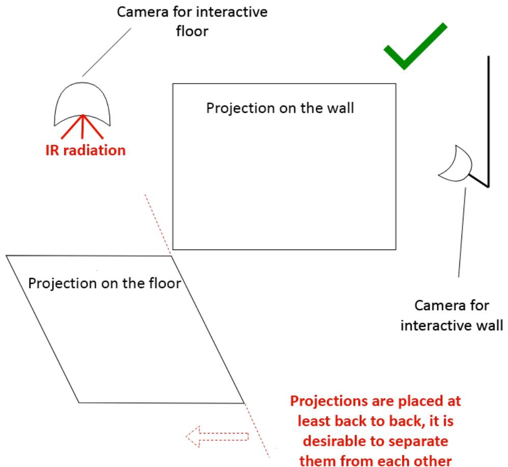
**Pic. 9 An example of the correct joint installation of the Interactive Floor and Interactive Wall systems**
