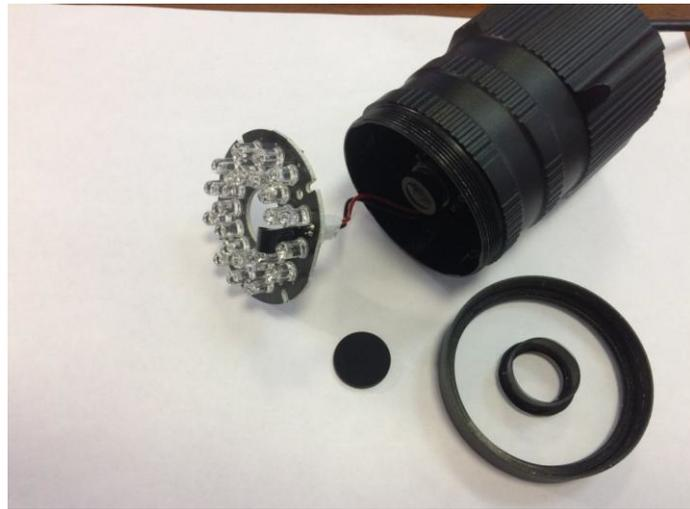
**Pic. 8 Example of an IR light source - CCTV camera with built-in IR illumination for an interactive floor**
