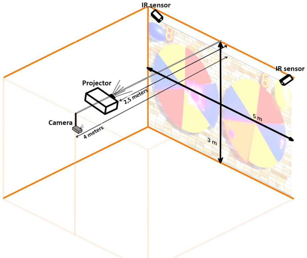
**Pic. 3 Recommendations for the installation of equipment elements**
