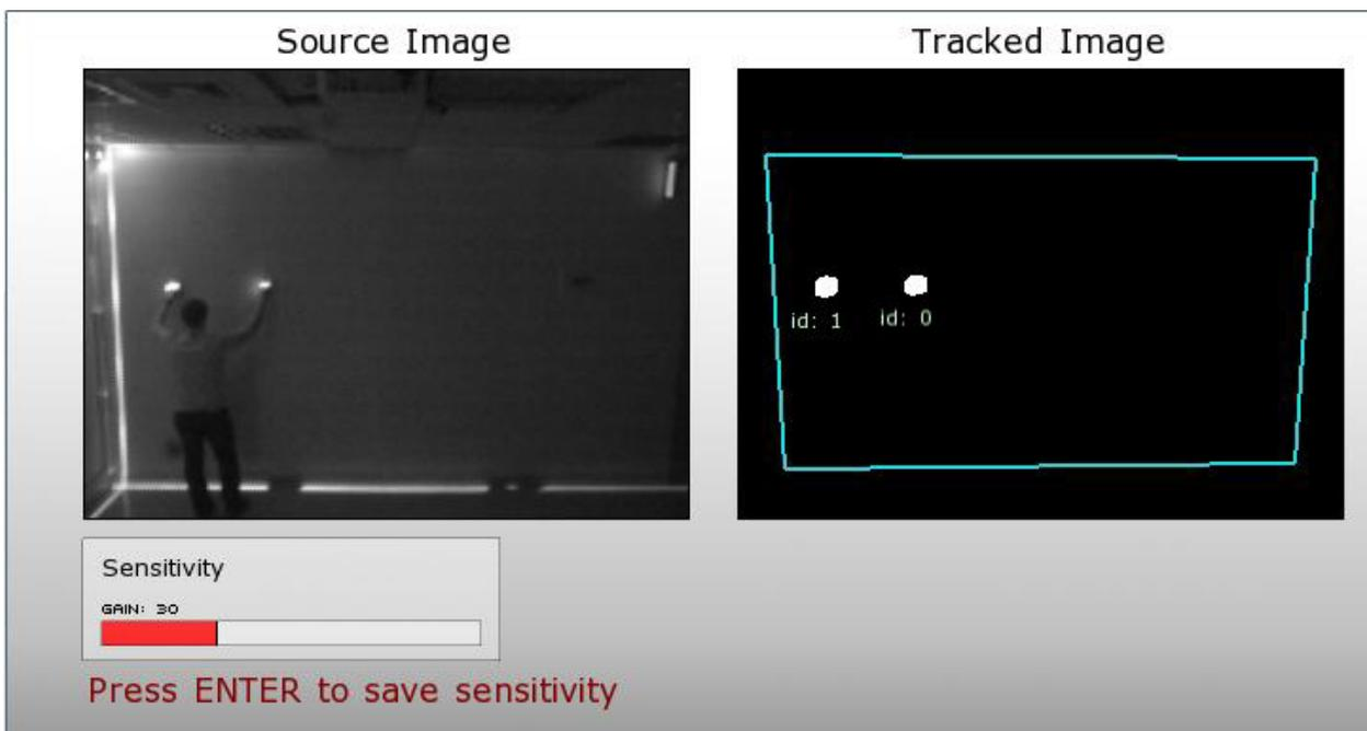
Pic. 30 Example of camera sensitivity setting (Gain is 30)
