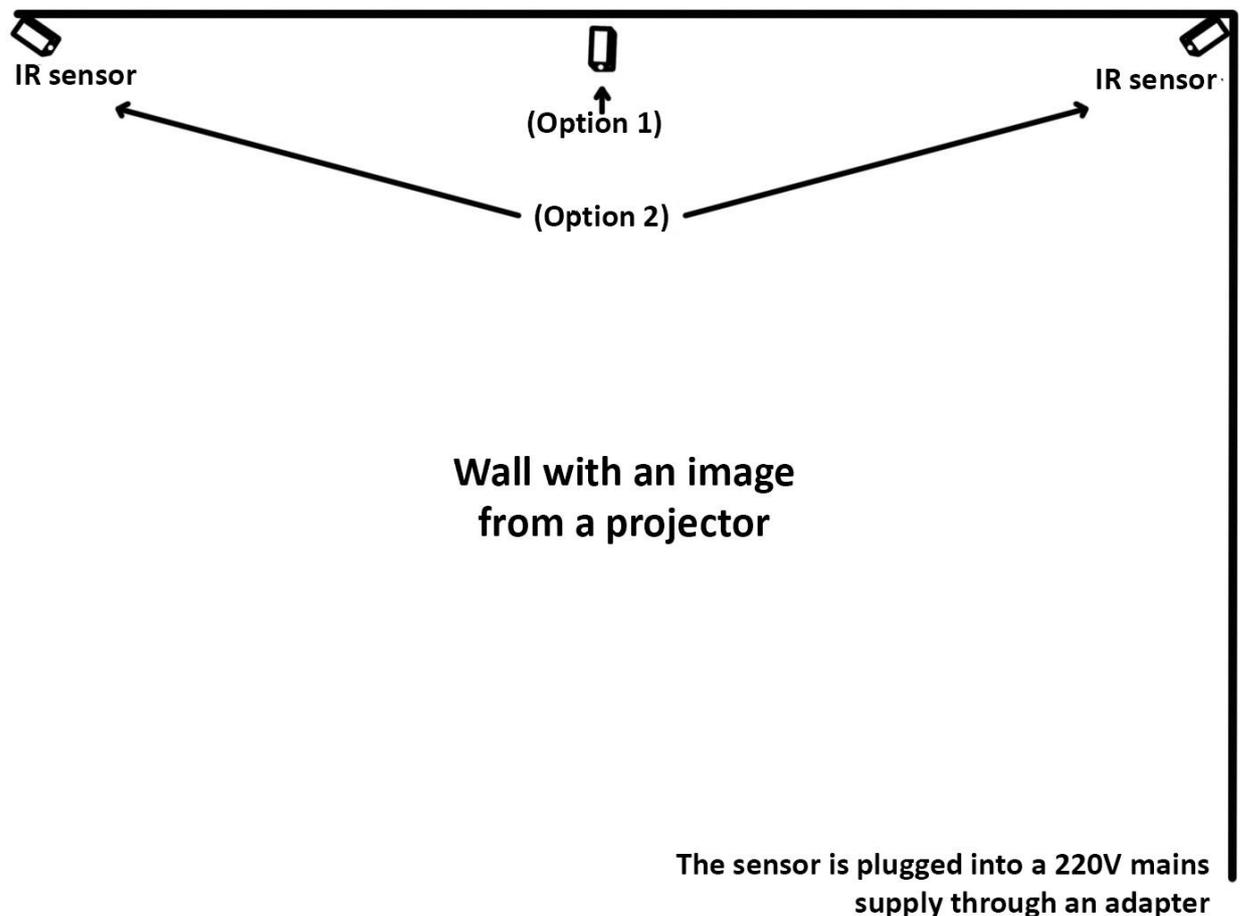
**Pic. 4 Infrared sensor placement options**
