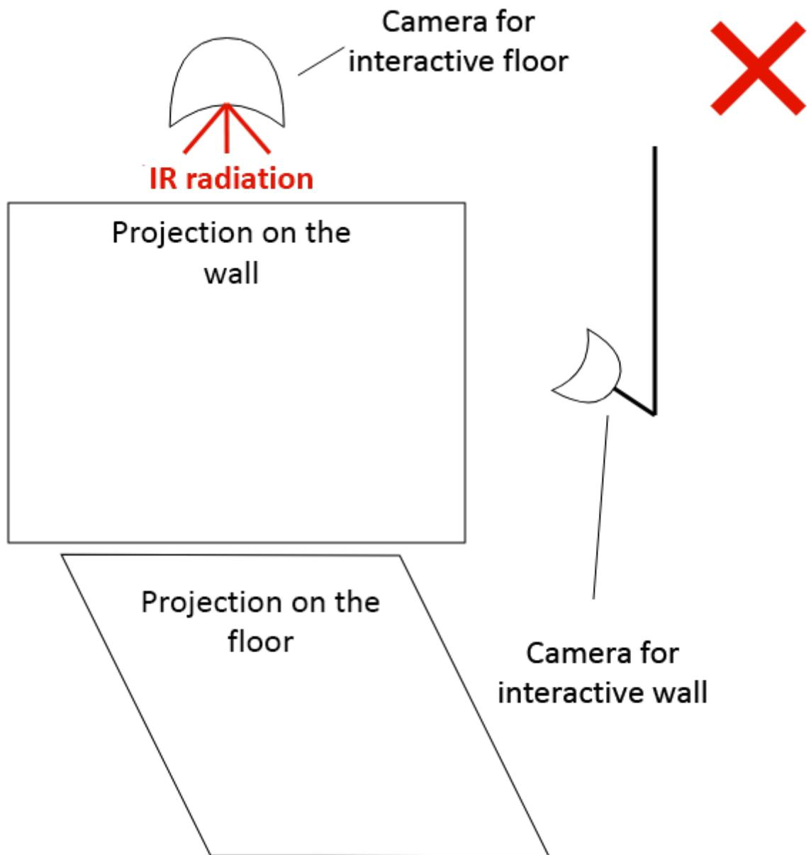
**Pic. 10 An example of incorrect joint installation of the Interactive Floor and Interactive Wall systems**
